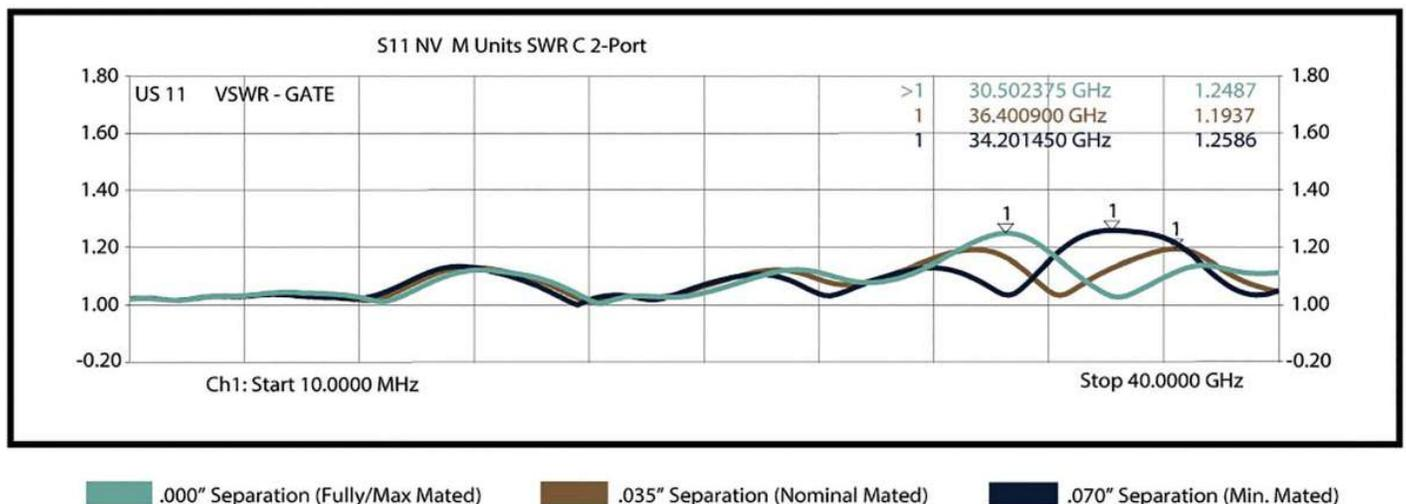
VSWR performance of a size 12 PkZ mated pair to 40 GHz at three stages of mating. Image: The Phoenix Company of Chicago
